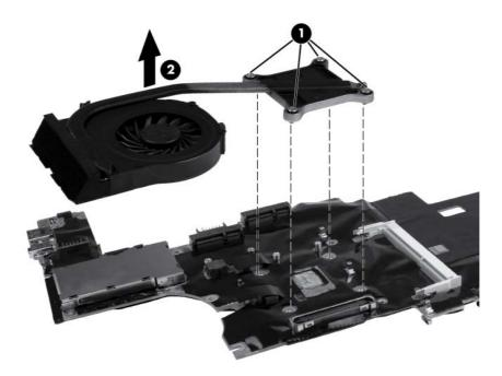
**NOTE:** The thermal material must be thoroughly cleaned from the surfaces of the heat sink (1) and processor (2) each time the heat sink is removed. Thermal material is included with fan/heat sink assembly and system board spare part kits.
